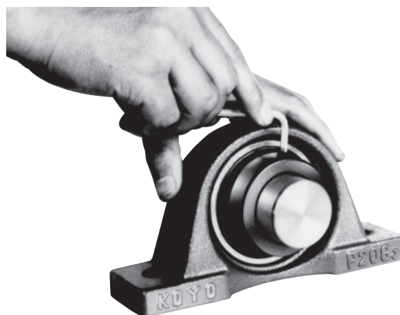
Fig. 14.10 Installing eccentric locking collar
